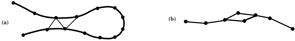
Figure 2: Problems encountered when connecting new vertices. (a) Connecting regions that fold back near one another. (b) “Bubbles” resulting from incorrect joining of vertices.
