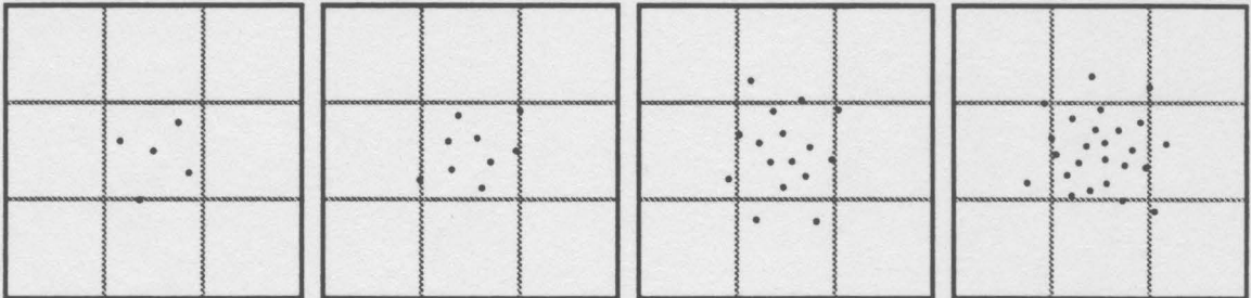
Figure 4: Kernels containing 5, 9, 16, and 25 samples.
