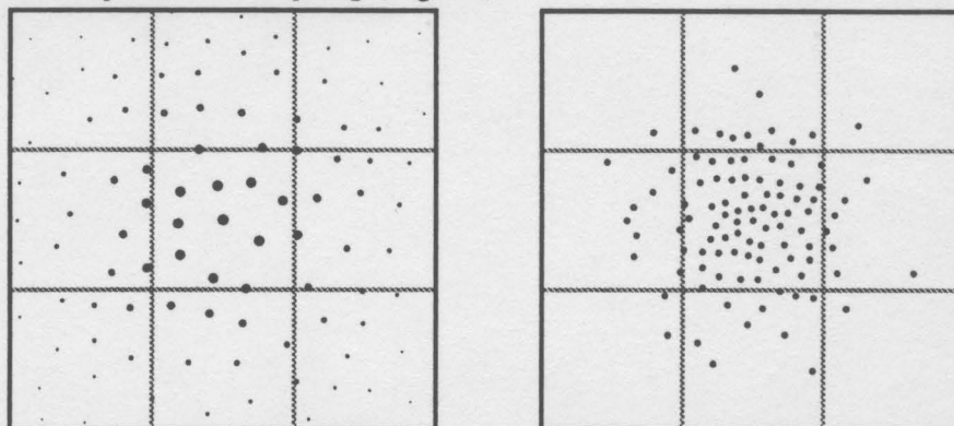
Figure 3: a) Uniform sampling with weighted samples and b) Importance sampling with unweighted samples.
