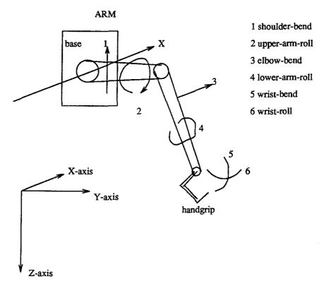
Figure A.1: The six ARM joints.
