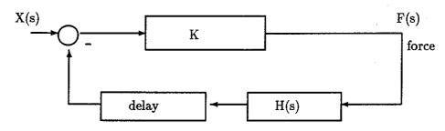
where K = spring constant,  $H(s) = 1/(Ms^2 + Bs)$ , M: mass, B:viscosity, delay =  $e^{sT}$ , T: sampling period
