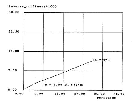
Figure 7.3: Joystick 1/stiffness (in m/N) versus sampling period (in ms).
