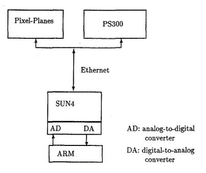
Figure 1.1: System configuration.
