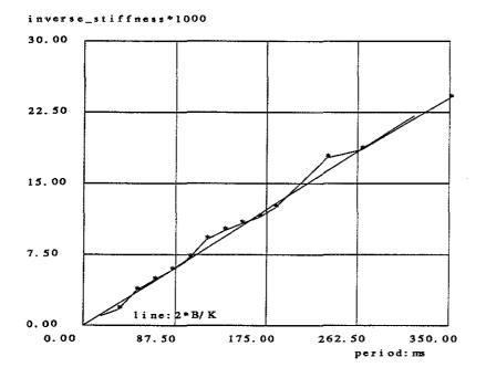
Figure 7.1: ARM's shoulder-rotation 1/stiffness (in m/N) versus sampling period (in ms).
