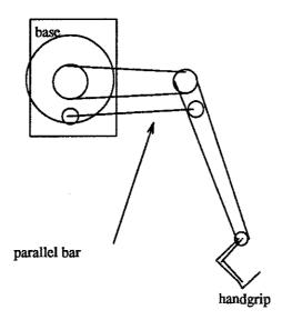
Figure A.2: The special elbow-bend joint with a parallel bar.
