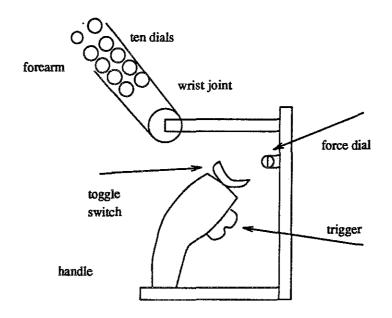
Figure 1.4: The side view of a modified hand-control at the wrist
