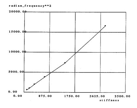
Figure 7.4: Joystick frequency squared (in radian) versus stiffness (in N/m).
