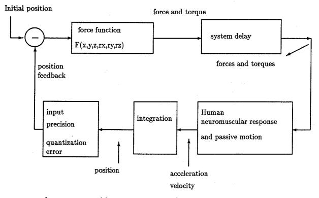
where x,y,z are positions, rx,ry,rz are rotations, F() is a force field function.
