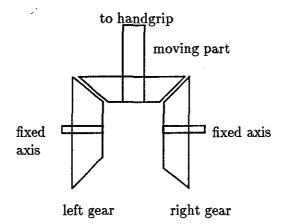
Figure 10.1: Differential gears at the ARM wrist joint.
