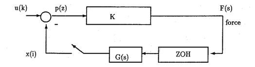
where G(s) = 1/[s(B + Ms)], M is the mass attached to the end of springs, B = viscosity, K is the stiffness of the springs, u(k) = initial position, x(i) = feedback position of handcontroller, p(z) = deviation from null position used in the spring force calculation, and ZOH is a zero-order-hold (sampleand-hold).
