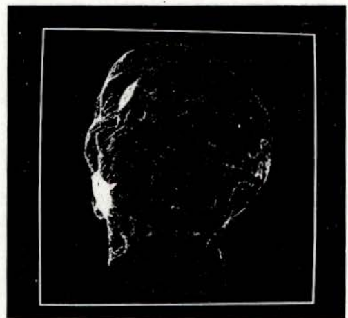
Figure 13: "Cost image" showing the computation expense at each pixel for generating Figure 12. In this case, the user-defined threshold for proceeding with Phong shading passed about 50% of the front-facing polygons.
