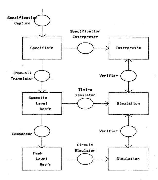
Figure 3-7. Role of Specification Interpreter in the VLSI Design Process.
