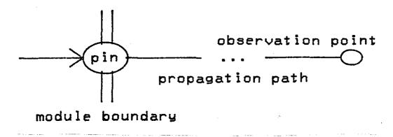
Figure 4-3. Canonical Test Environment.
