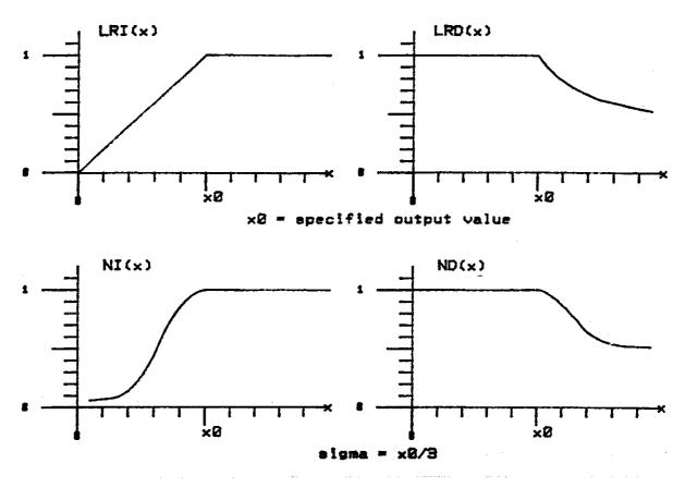
Figure 4-2. Linear Ramp (LR) and Normal (N)
