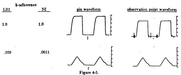
Change Propagation through a Steered Signal Path in nMOS.
