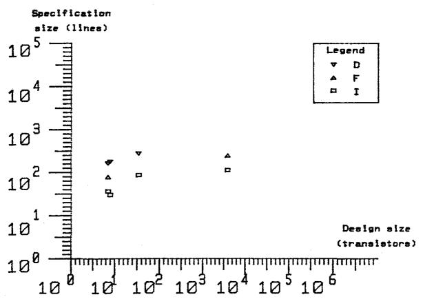
Figure 4-1. Scalability of Proposed Specification Method. (See text for legend.)
