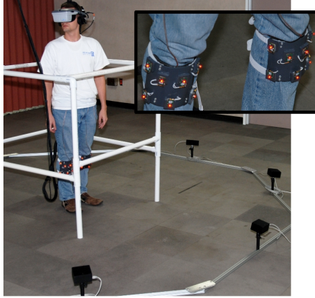
Figure 2.12: A user in the UNC GUD WIP system: The user wears beacons for 6-DOF trackers on his shins (inset). Beacon-tracking cameras surround the subject on the floor. The heel’s position is approximated by rigid-body transform from the shin’s pose.
