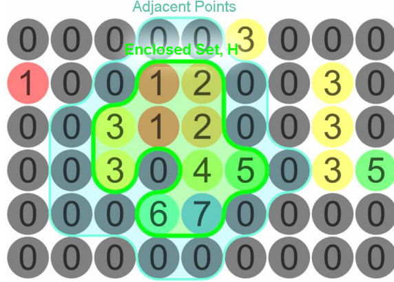
Figure 3.2: A set of points H is enclosed by empty space. Every point adjacent to H is labeled zero and the zero label is adjacent to itself in all directions T_x(0,0) = T_y(0,0) = 1 .
