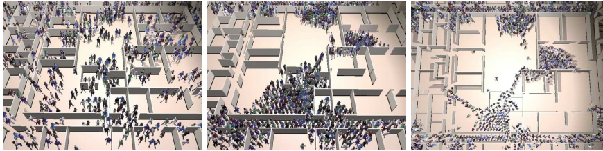
Fig. 9 Snapshots from simulation of 1,000 virtual agents evacuating an office as part of a crowd simulation.
