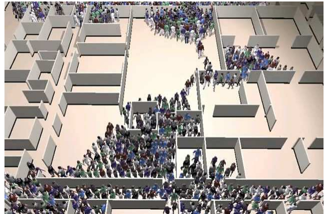
Figure 1: Building evacuation: 1,000 independent agents in different rooms of a building move towards the two exit signs and cause congestion. P-ClearPath can efficiently perform local collision avoidance for all agents in such tight packed simulations at 550 FPS on Intel quad-core Xeon (3.16GHz) processor. Our algorithm is more than an order of magnitude faster than prior velocity-obstacle based algorithms.
