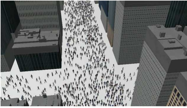
Figure 6: Urban simulation: 25K independent agents walking in a city model on sidewalks and intersections. P-ClearPath can efficiently perform local collision avoidance for all agents in this simulation at 20 fps on Intel quad-core Xeon (3.14GHz) processor
