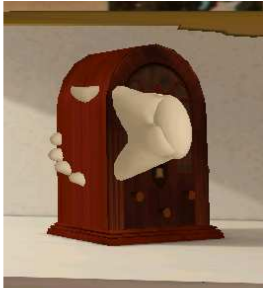
Figure 1-1. Interpenetration problem: A user may see his hand avatar penetrate a virtual object when the object he is reaching for does not exist in the real world.
