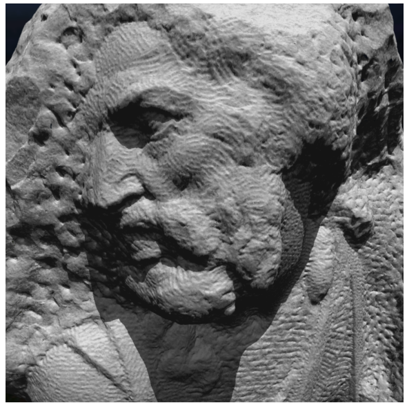
Figure 11: St. Matthew model with shadows. This image shows St. Matthew model consisting of 372 million triangles. We are able to render the model with high quality shadows at 15-25 frames per second on commodity hardware with a GeForce 7800 GTX GPU.
