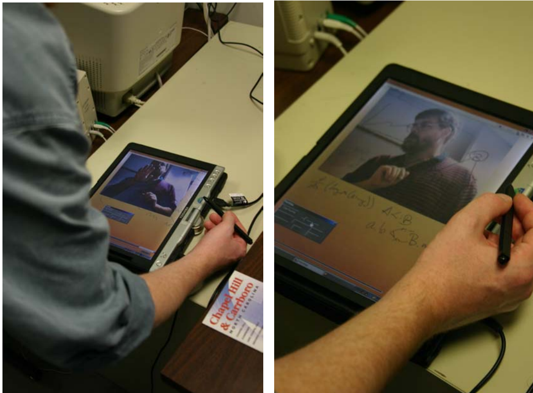
Figure 6: Note taking on top of interpreter's semi-transparent video image
