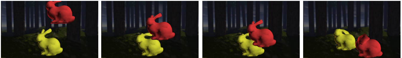
Figure C.1: Proximity Computations on Deforming Models: We use our interactive distance field computation for separation and penetration distance for dynamic simulation of deforming bunnies. Each bunny consists of 2K triangles and we compute localized distance fields on a 256^3 grid for the simulation shown in this sequence. The average distance field and proximity query takes 120ms on a 3.2 GHz Pentium IV PC with NVIDIA GeForce 7800 GPU.
