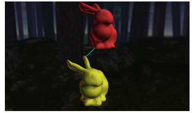
Figure 3: Separation Distance Computation between deforming bunnies: Average query time=120ms, grid resolution= 256^3 .
