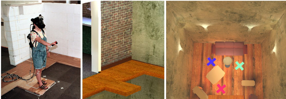
Figure 1.11 - The virtual pit scene. Left: A photograph of the real world. The user knows there is a real floor. Center: view of the virtual scene. Right: The virtual scene from the user's viewpoint.
