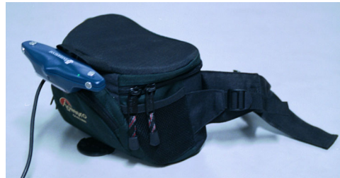
Figure 8.3 - The hand-tracking sensor attached to a hip-worn camera bag in order to track the torso orientation.
