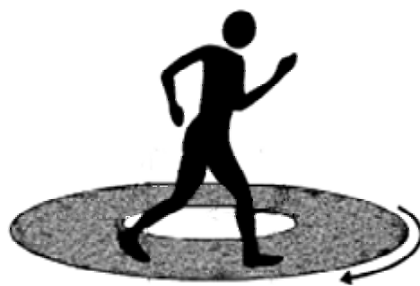
Figure 4.9 - The rotating treadmill used by Gordon et al. The disk was 5 ft in diameter and spun at 22 deg/s. Subjects walked around the disk such that they stayed in the same spot while the disk turned underneath them [adapted from Gordon 1995].
