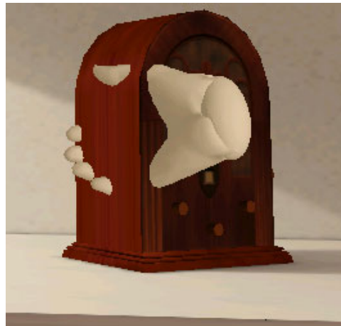
Figure 11.1 - The user's tracked virtual hand penetrates the virtual antique radio [from Burns 2003].
