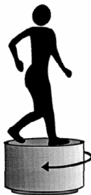
Figure 4.10 - The rotating turntable used by Weber et al. Subjects walked in place while the turntable spun beneath them [adapted from Weber 1998].
