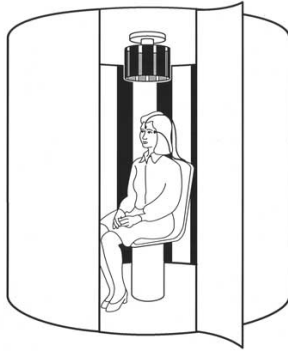
Figure 4.12 - An optokinetic drum, where the person is seated on a stationary chair while the surface of the drum, which has alternating vertical stripes painted on it, rotates about the person [from Hain 2005]
