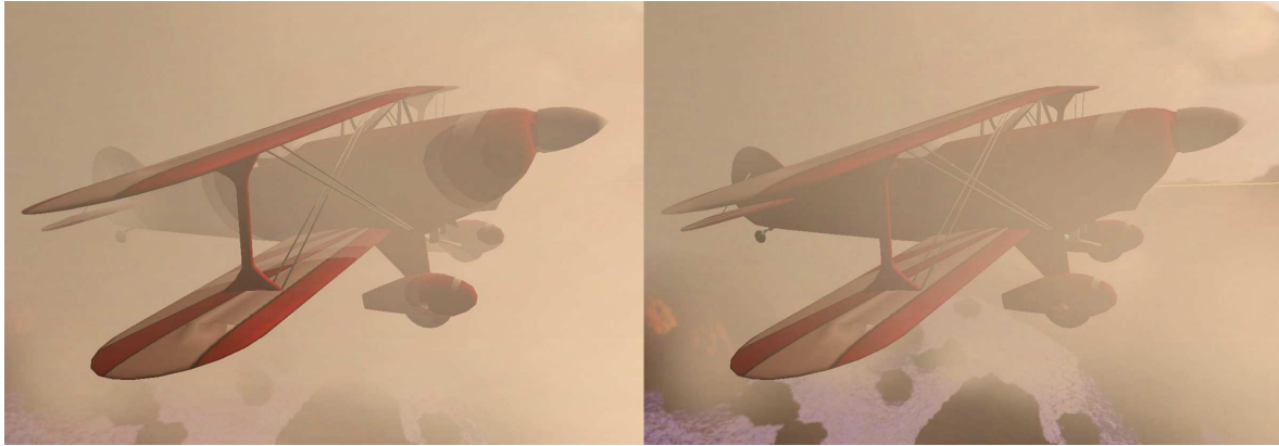
Figure 6.10: An airplane in the clouds. Left: particles directly rendered into the scene cause visible artifacts where the particle geometry intersects the airplane geometry. Right: impostor splitting removes the artifacts, because the airplane is composited between two impostor layers without depth testing.
