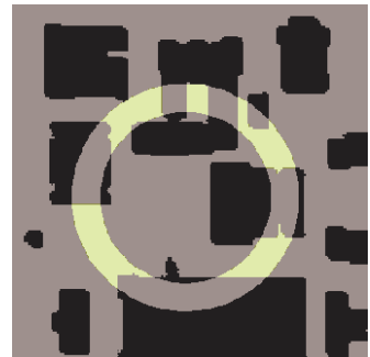
Figure 2: Example of the usage of an outdoors map to filter out the regions where a host cannot be located.
