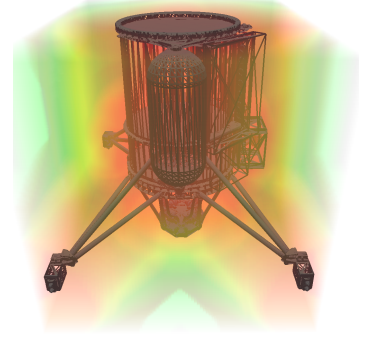
Figure 8. Cassini Model: A volume rendering of the distance field of the Cassini with 93K polygons. The distance to the surface is color coded, increasing from red to green to blue.
