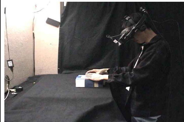
Figure 26 – Visually Faithful Hybrid Environment (VFHE) setup. Participants manipulated real objects and were presented with a visually faithful avatar.
