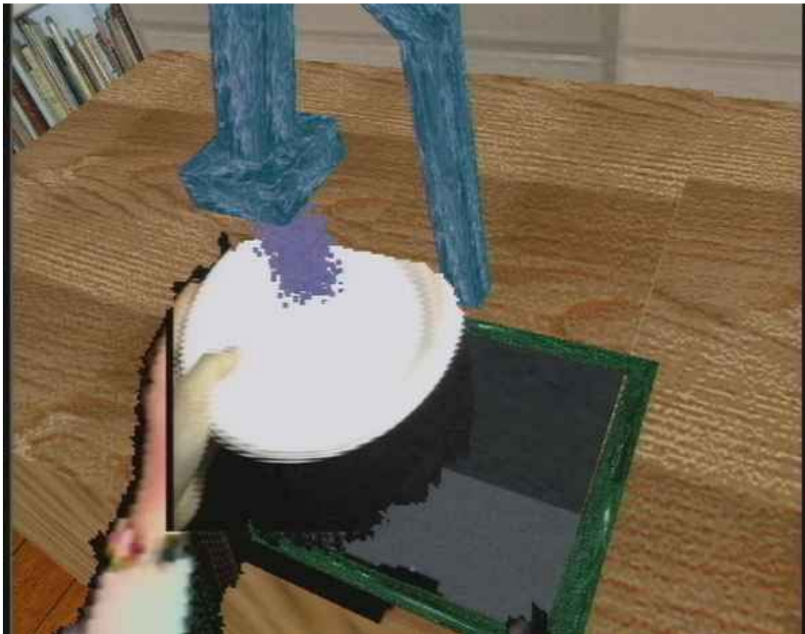
Figure 18 – The real-object avatars of the plate and user are passed to the particle system as a collision surface. The hand and plate cast shadows in the VE and can interact with the water particles.
