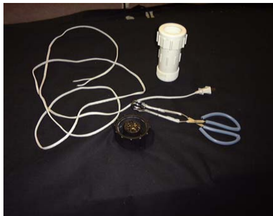
Figure 38 – Parts used in the shield fitting experiment. PVC pipe prop, power cord, tongs (tool), and the outlet and pipe connector that was registered with the virtual model.
