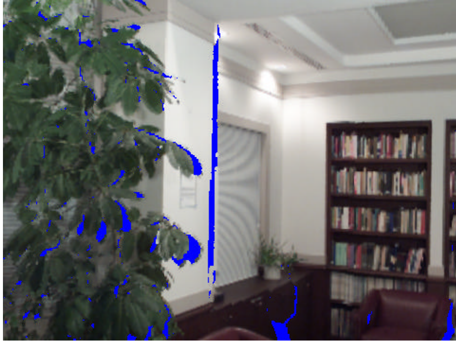
Figure 1-1:: Disocclusion artifacts of 3D Image Warping (shown in the blue background color).
