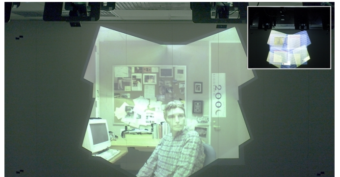
Figure 13: PixelFlex in a stacked configuration where four of the projectors almost entirely overlap the other four projectors. This demonstrates that the algorithm is capable of supporting stereo display configurations in the future. The inset shows the rough projector alignment.
