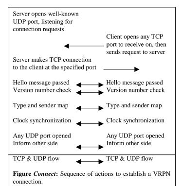
verification"). When the server receives the connection request, it opens a new communications endpoint, which calls the client back at its specified TCP port.
