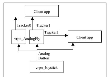
**Figure** *Layered*: Devices can be layered, so that the outputs from one device driver can become inputs to another. Application code can attach to either or both devices. The same driver can export multiple interfaces of the same type under different names.
