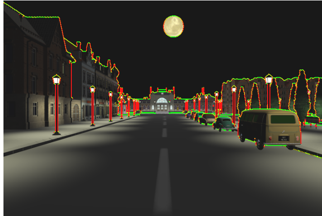
Figure 1.2 Depth-discontinuity detection in the reference image. The vertical and horizontal depth discontinuities are marked in green and red, respectively. On black and white copies the depth discontinuities appear as lighter pixels at silhouettes. The detection algorithm works well in spite of the great range of distances in the image.
