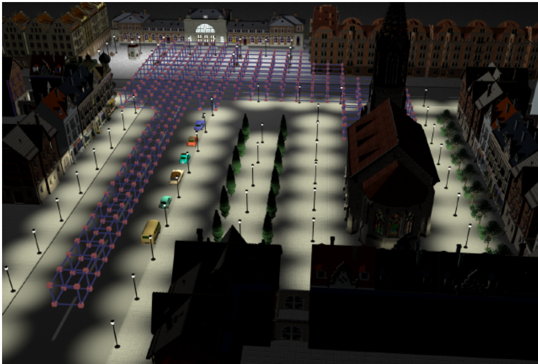
Figure 5.7. Overview of the Eurotown scene. The little solid (pink) cubes indicate the sampling locations from which the depth and color panoramas were acquired. A panorama consists of 6 depth images with 90 degree horizontal and vertical fields of view that correspond to the faces of a cube. The depth images are 1K x 1K in the case of VGA output (70 deg horizontal field of view) and 2.8K x 2.8K in the case of HDTV (70 deg FOV). The total space consumed by all of the depth images is 4.33GB and 26.06GB respectively, with lossless RLA compression. The wire-frame defines the cells that subdivide the viewing volume.
